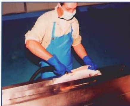
Using Jarvis' CV-1 to extract salmon blood lines at the Aquatas Tasmania fish processing plant in Margate, Tasmania.
