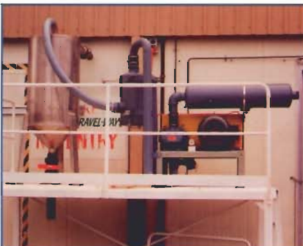
Picture of the vacuum tank setup at Aquatas' Margate, Tasmania plant. Built to customer specifications, the system has a 15 hp lobe vacuum pump, an 80 gallon cyclone type stainless steel tank and four lung gun type wands.
